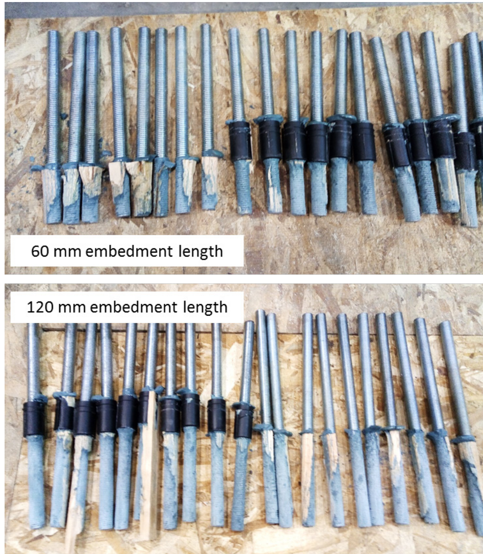
Figure 3 Examples of rod withdrawal failure
